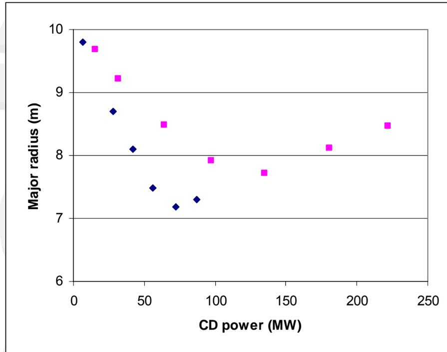
Reducing  $\gamma_{CD}$  by a factor of 5 changes results but still full non-inductive plant is smaller than full inductive. Possible optimum at less than full CD but this is not a proper comparison of pulsed vs steady-state. It is **not true** that steady state plants cannot be built using less efficient CD systems.
