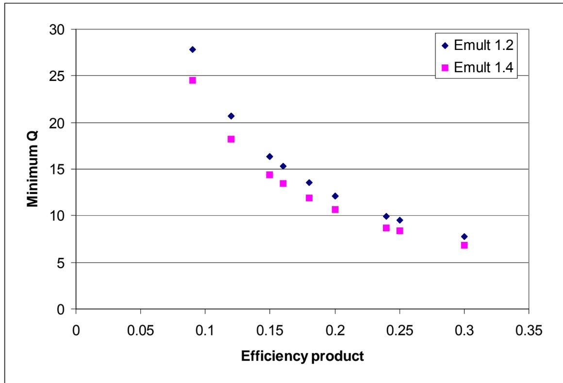
Efficiency product multiplies CD wall plug efficiency and plant electrical conversion efficiency.
