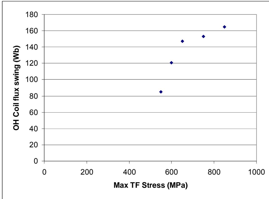
OH coil size can be substantially changed by relatively small change in allowable TF stress
