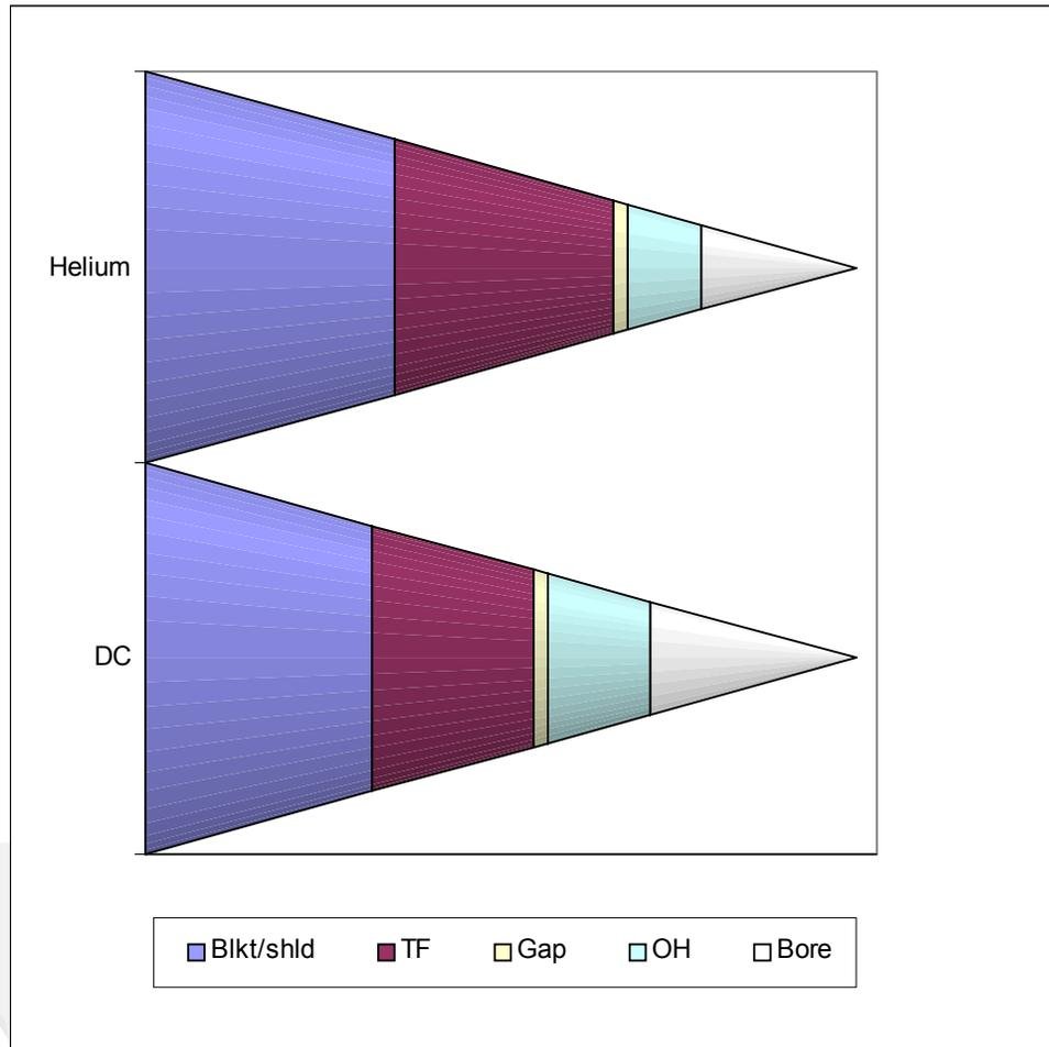
Potential for reduced OH coil size with helium coolant than with Dual Coolant concept. This is only an example.
