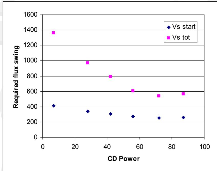
Current drive sustains some of the current reducing the voltage requirements and reduces the required flux swing
