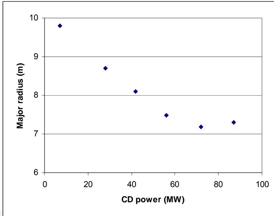
Major radius is substantially reduced by adding CD power (here 2 MeV NNBI, but what if lower CD efficiency?).
