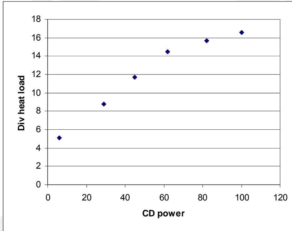
Increasing CD power reduces size (cost) and increases power density. This is not heading to an optimum steady state plant as the basic assumptions are still characteristic of a pulsed plant (aspect ratio, energy storage...)
