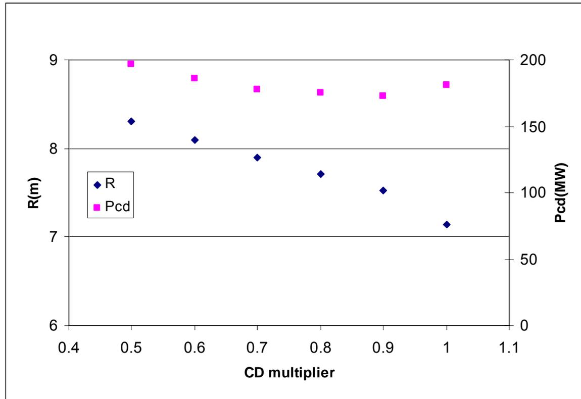
Reduce CD efficiency by a multiplier. Design optimisation changes size (and  $q$  and bootstrap fraction) to avoid excessive CD Power. Self consistent plant couples changes and outcomes often non-intuitive.
